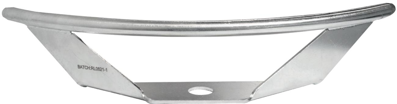
The Intermediate 90° is designed to be installed on the Cone. It is a cable support used on sharp corners. Due to the design the shuttle can easily slide over the it without disconnecting it from the lifeline.
