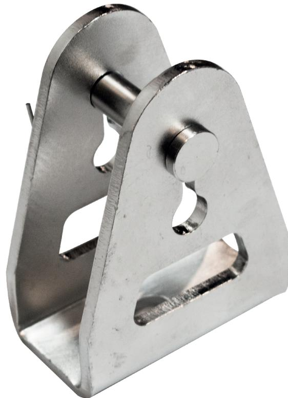
The End Point is the connection between the line system and the structure. It is designed for easy installation on steel/concrete beams and structures of sufficient strength. The End Point is designed to rotate and always be in line with the cable, which results in minimal shear stress in case of a fall.
