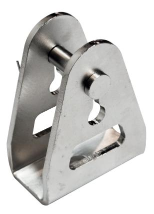
The End Point is the connection between the line system and the structure. It is designed for easy installation on steel/concrete beams and structures of sufficient strength. The End Point is designed to rotate and always be in line with the cable, which results in minimal shear stress in case of a fall.
