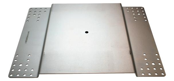
The Square Base Plate 500 for metal profile roof panels and standing seam roofs is designed for installation and attachment on the roof surface, in this way the integrity of the roof is protected. The Square Base Plate 500 can be fixed with clamps on standing seam roofs or with rivets on metal roof panels.
