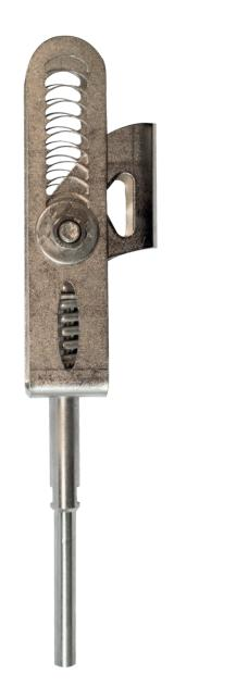
The Vertical Shock Absorber is installed at the top bracket of the system. The product absorbs the energy of the fall and limits the damage to structures, it is developed to act according to the principle of Instant Energy Absorption (IEA) significantly reducing the force on the lifeline in case of a fall. The absorber also works as a tensioner and has a tension indicator.
