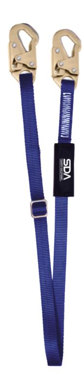
Positioning lanyard made of high tenacity polyester webbing. 6ft. (1.8m) length, with  $2 \times 3/4$ " steel hooks.
