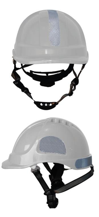
Type II helmets for work at heights, confined and/or electrical spaces, and industry in general, made of ABS thermoplastic with high resistance to lateral and vertical impacts. It has a Ratchet system for graduated 6-point tape adjustment and a reflective band
