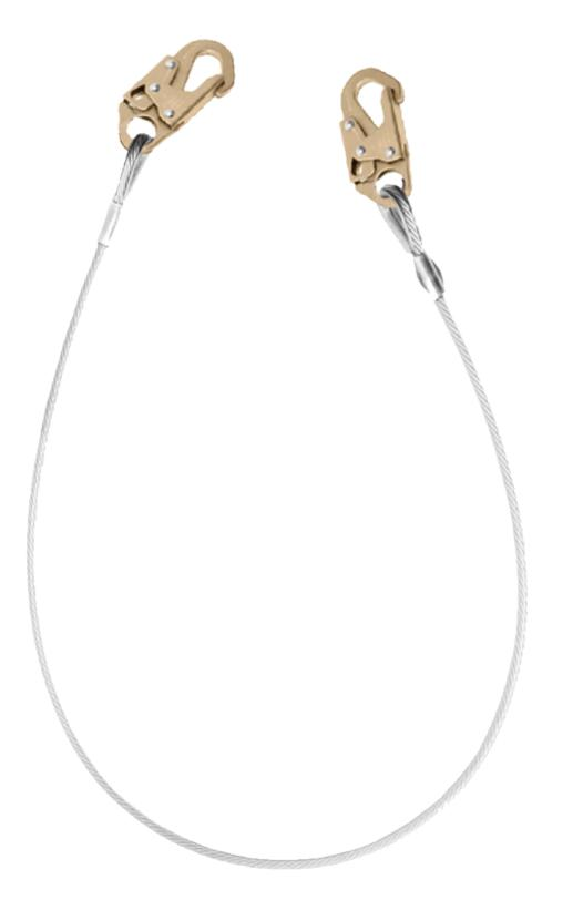
Positioning lanyard made of steel 1/4" (6mm) cable. 6ft. (1.8m) length, with 2 x 3/4" steel hooks.
