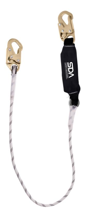
Fall protection lanyard made of high tenacity polyamide Kernmantle rope 7/16" (11mm). 6ft. (1.8m) length, with 2 x 3/4" steel hooks.
