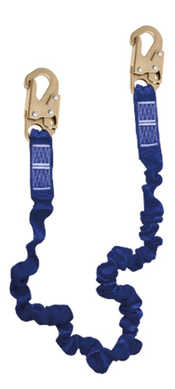
Fall protection lanyard made of high tenacity polyester webbing. 6ft. (1.8m) length, with  $2 \times 3/4$ " steel hooks and integrated absorber.
