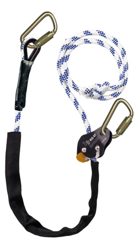
Positioning lanyard made of high tenacity polyamide Kernmantle rope 7/16" (11mm). 6ft. (1.8m) length, with  $2 \times 3/4$ " steel twist-lock carabiners.
