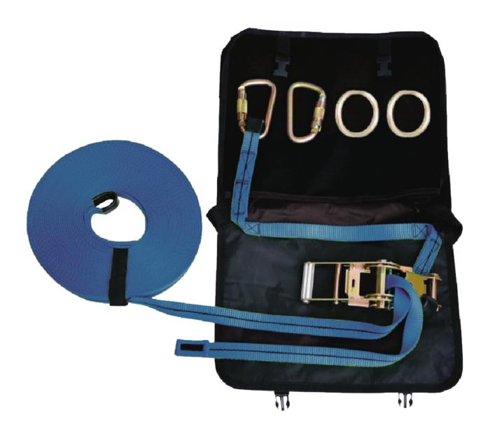
The temporary horizontal webbing lifeline can be adjusted from 6.5 to 65.6 ft (2 to 20 m). It can be connected to an anchor strap and the ratchet is used to provide the tension to the system after setting the distance required. Suitable for two persons at the time.
