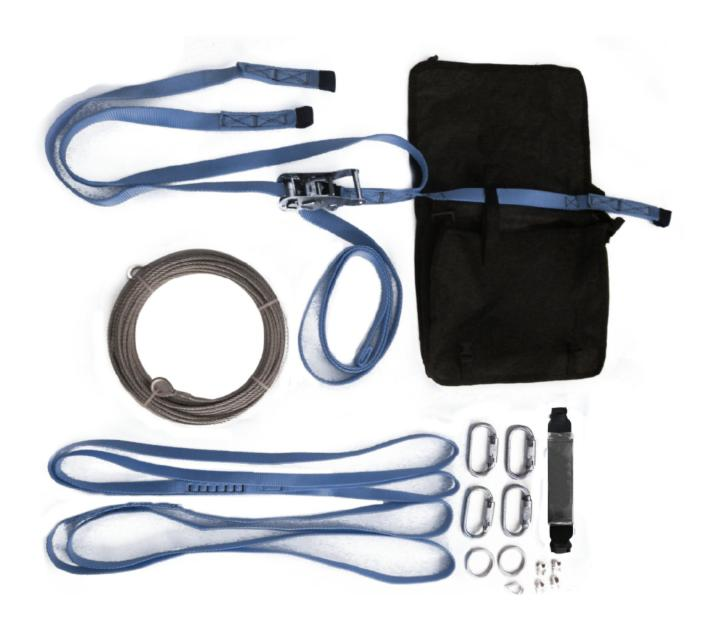
The temporary horizontal cable lifeline can be adjusted from 6.5 to 65.6 ft (2 to 22.5 m) and keeps the user insured during their displacements. It can be tied to an anchorage connector. The ratchet is used to give tension to the line after setting the required distance. Suitable for the use of 2 persons.
