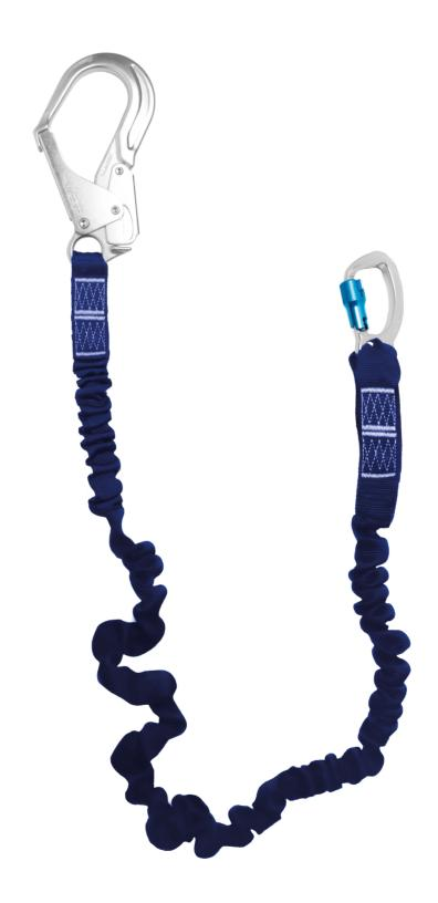
Fall protection lanyard made of high tenacity polyester webbing. 6ft. (1.8m) length, with 1 x 3/4" & 1 x 2 1/4" aluminum twist-lock hooks and integrated absorbers.
