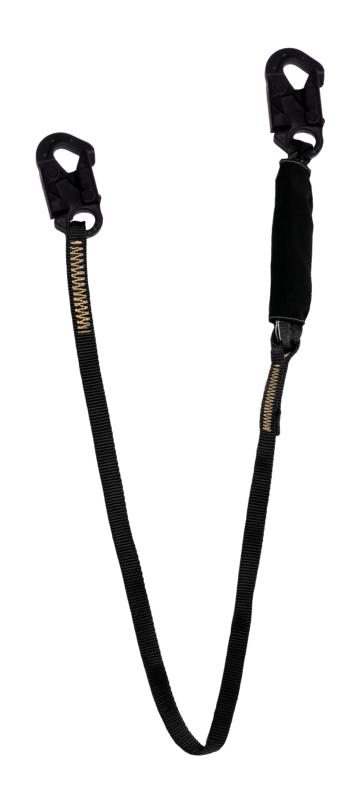
Fall protection lanyard made of Aramid webbing. 6ft. (1.8m) length, with 2 x 3/4" dielectric hooks, and aramid absorber sleeve.
