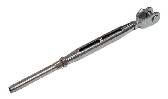
The Tensioner is designed to be the permanent interconnection between the cable and the End Points. It has a tension adjustment system that works by rotation and is blocked with locking nuts once the desired tension is reached.
