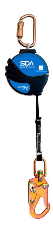
High-impact strength Polymer Housing with Dyneema (UHMPE) webbing, and a steel swivel hook.  $5.5" \times 3" / 14.2 \text{ cm } \times 7.7 \text{ cm}$  size, 20 ft / 6 m length webbing.
