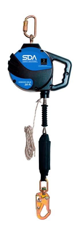
High-impact strength Polymer Housing with carry handle, stainless steel cable, and a steel swivel hook.  $8.3" \times 4.7"/21.1$  cm x 12.1 cm size, 20 ft / 6 m length cable.
