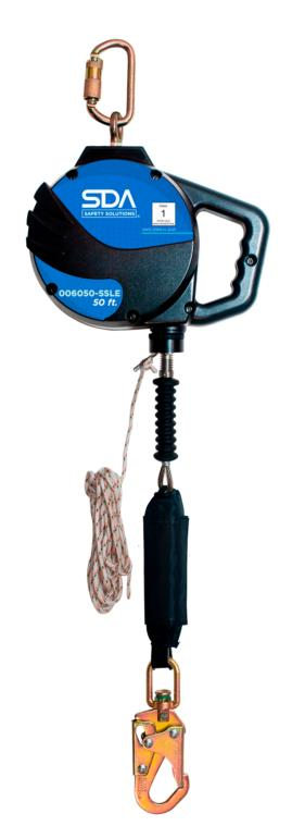
High impact polymer housing with stainless steel cable, and a steel swivel hook. 9.6" x 4.7" / 24.5 cm x 12.1 cm size, 50 ft / 15 m length cable.
