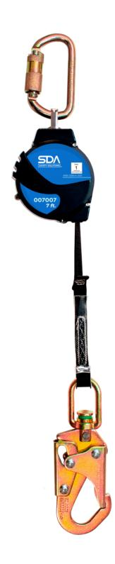
High-impact strength Polymer Housing with Dyneema (UHMPE) webbing, and a steel swivel hook.  $2.83" \times 4.4" / 7.2 \text{ cm} \times 11.3 \text{ cm}$  size, 7 ft / 2 m length webbing.
